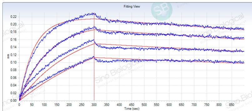
Loaded Human ACE2 Protein (hFc tag) (Cat. No. 10108-H02H) on AHC Biosensor, can bind SARS-CoV-2/2019-nCoV Spike/RBD Protein (RBD, mFc Tag) (Cat. No. 40592-V05H) with an affinity constant of 0.34 nM as determined by Octet RED System.
